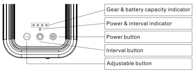
①Press the power button ② to turn on the air pump. The green indicator light will illuminate. Press the power button again to turn off the air pump. The green indicator light will turn off.
