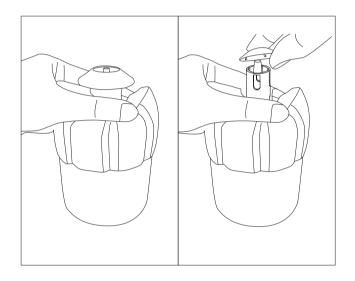
**Step2.** Two bio sponges are pre-installed in the filter. To use, please remove one.
