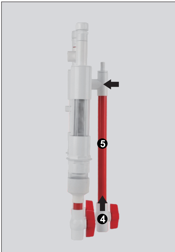
Step 3: Attach the connection with the valve ④ to the outlet pipe, and install the outlet pipe ⑤ to the lower tee connection of the filter body ①
